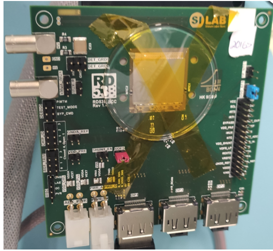
Fig. 52: A Single-Chip-Card with a CROCv1 chip without a sensor under a protective glass.
